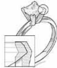
V-prongs are generally used for diamond shapes with points -- such as the corners of the square **Princess Cut** or the tip of the **pear shaped diamond**. The v-prong provides additional protection to the points which are often thin, fragile, and subject to chipping if left exposed.
