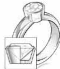
This simple change suddenly opens up the setting and gives it a totally modern look. The technique may also be used on a fancy cut diamond -- with an arc of precious metal around the wide curve of a pear shape and another, V-shaped section of precious metal embracing the narrow end.
