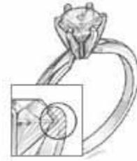
This is obviously a delicate balancing act. The more metal used to hold the diamonds, the more secure they are; the less metal used, the greater the chance for the diamond to reflect light.
